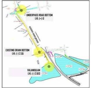
Level Difference - 2.6 m (Between underpass & valankulam) Distance - 1500 m Possible slope - 1:600 only
